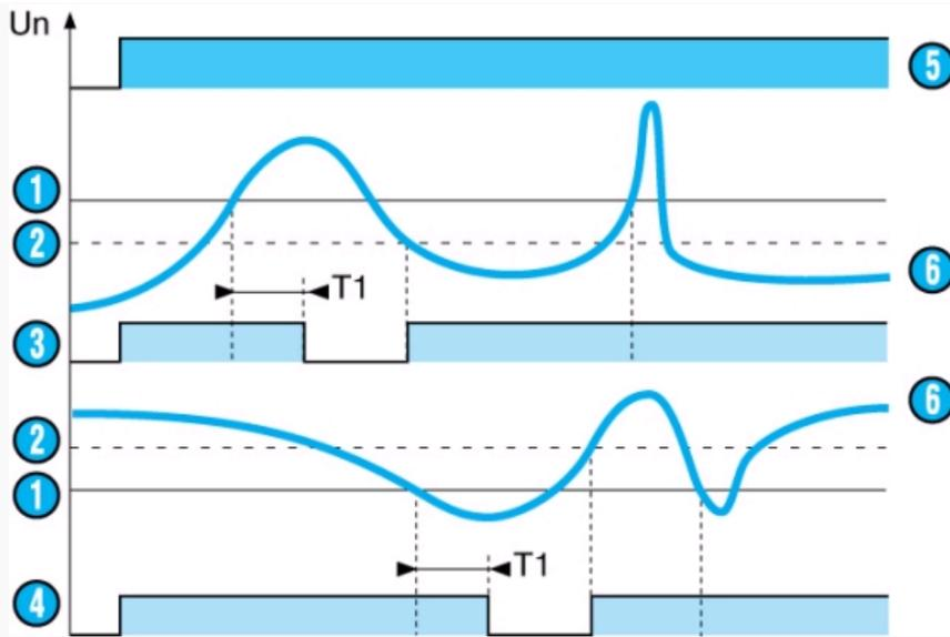
When the value of the controlled voltage, AC or DC, reaches the threshold  $U_e$  displayed on the front face, the output relay changes state at the end of a time delay  $T_1$ , which can be set on the front face at between 0.1 and 3s and remains latched in this position.
