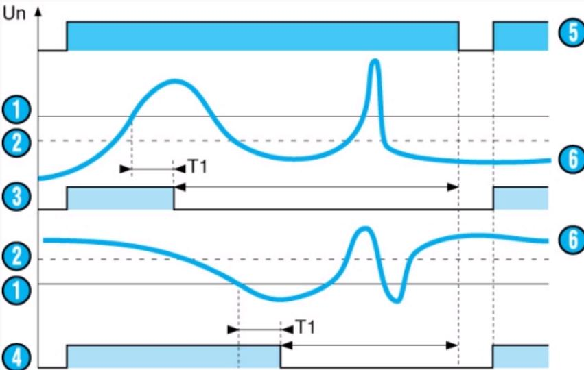
When the value of the controlled voltage, AC or DC, reaches the threshold  $U_e$  displayed on the front face, the output relay changes state at the end of a time delay  $T_1$ , which can be set on the front face at between 0.1 and 3s.
